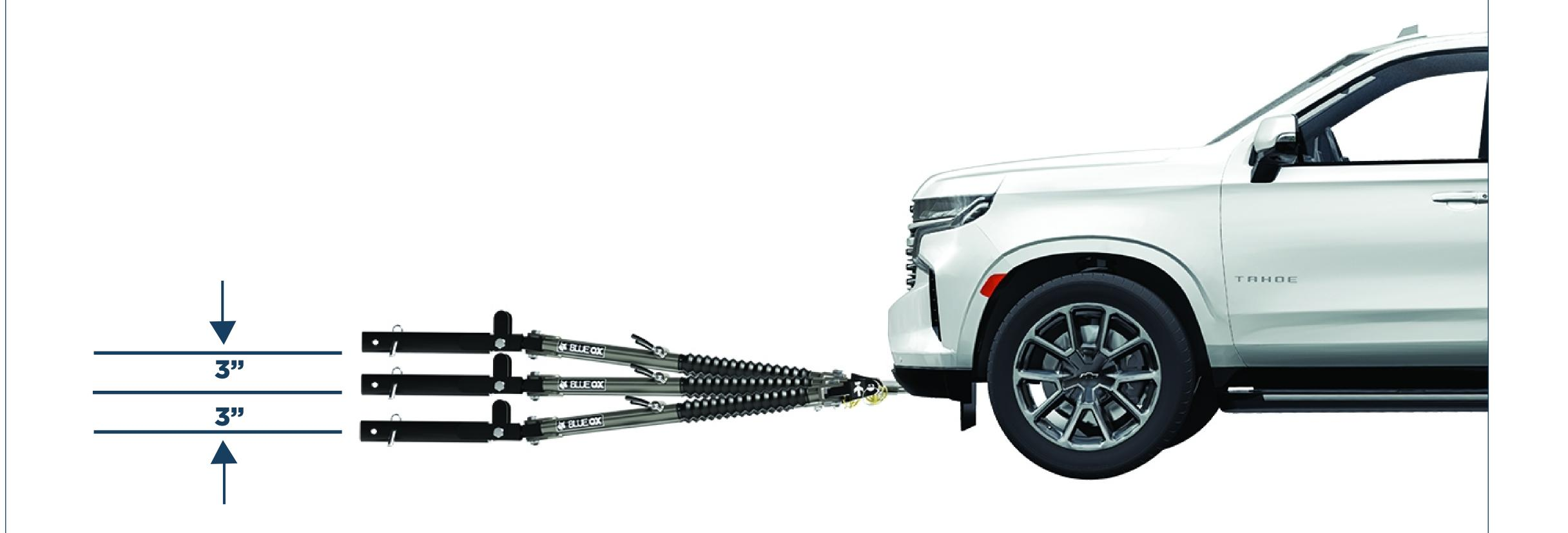
• SEAMLESS OPERATION OF THE TOW BAR HAPPENS WHEN THE TOW BAR IS +/- 3" FROM LEVEL WHEN TOWING. ADJUSTABLE RISE/DROP MAY BE NEEDED
